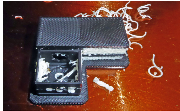
Fig. 9: Printing Result Some strings after half time printing but well PVA infilling!
